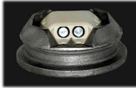
The invention consisted of glass beads sitting in a block of rubber on a metal base which was recessed into the road - even if vehicles drove over it the glass beads would drop down below the road surface undamaged. The idea took several years to ensure that *Cat's Eyes* could withstand all weathers and heavy traffic, and in 1937 Percy won a contract from the government for his invention.
